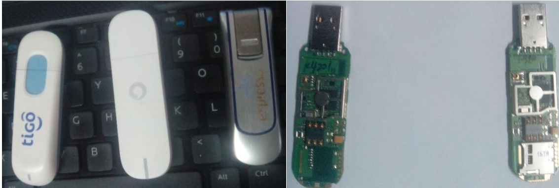
Figure 3: Huawei E303s-1, E303s-2, and EC167 (left) and E303s-1 and E303s-2 without external covers (right)
