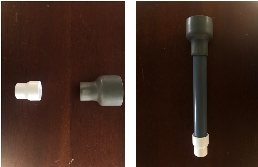
Figure 4. Reducers before and after being connected with a 1-inch pipe
