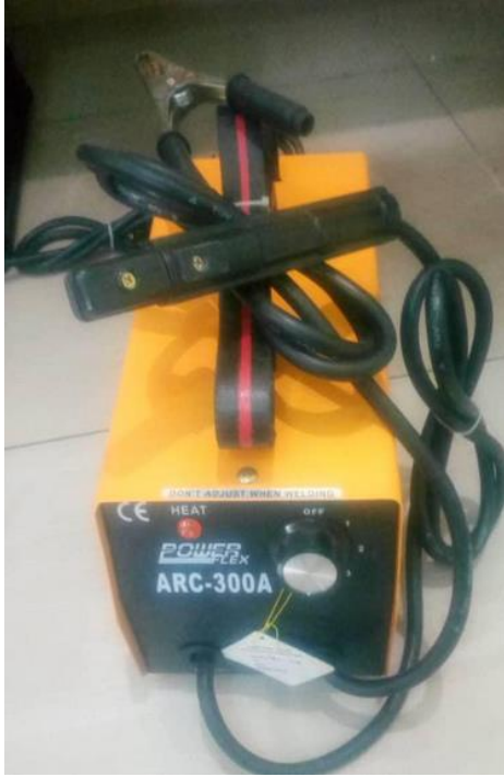
Figure 2: Welding machine used for welding steel frame together.
