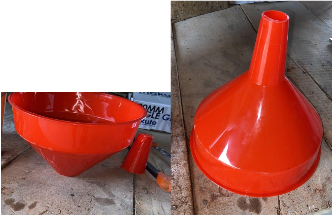
Figure 1: Conical funnel used for moulding the ceramic filter.
