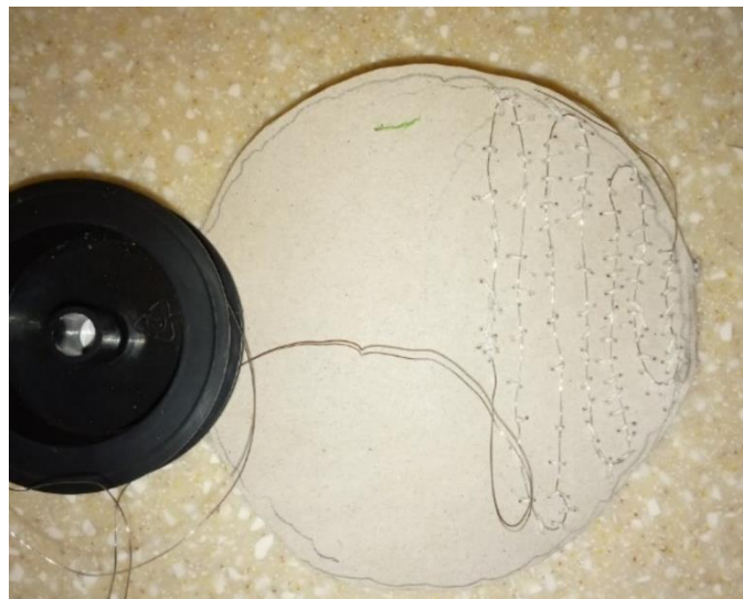
Figure 3.4: An image of the nichrome wire being sewn unto the paper
