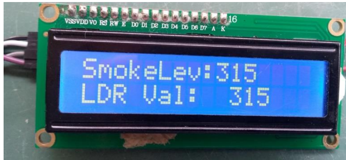
Figure 4.4: A display of the smoke level and Light Dependent Resistor value
