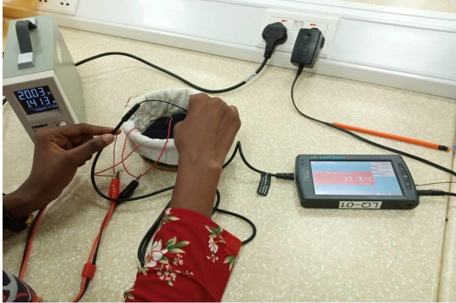
Figure 4.8: Reading temperature values from the surface of the mattress.
