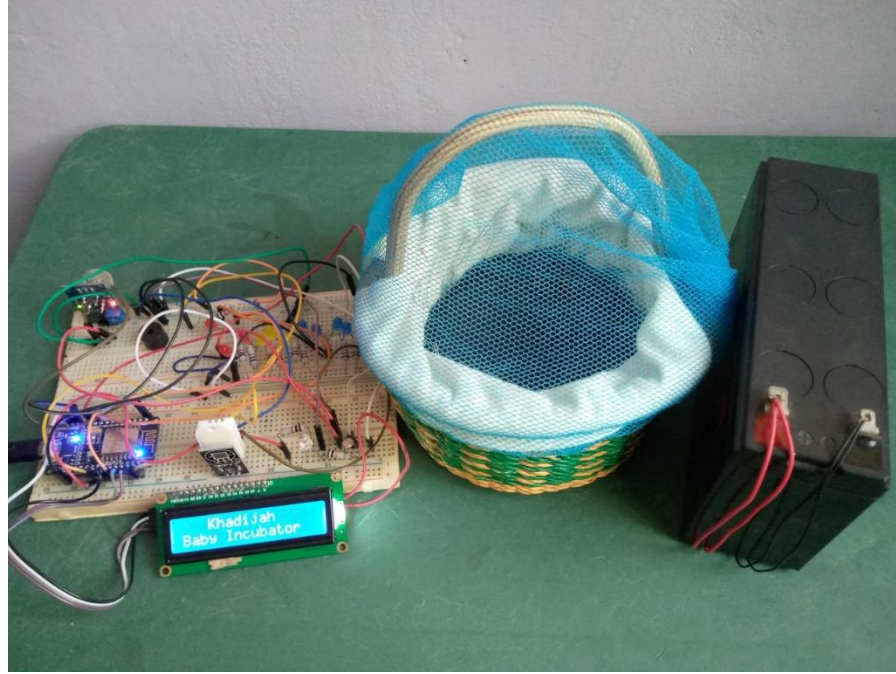
Figure 4.13: Overall hardware of the proposed solution
