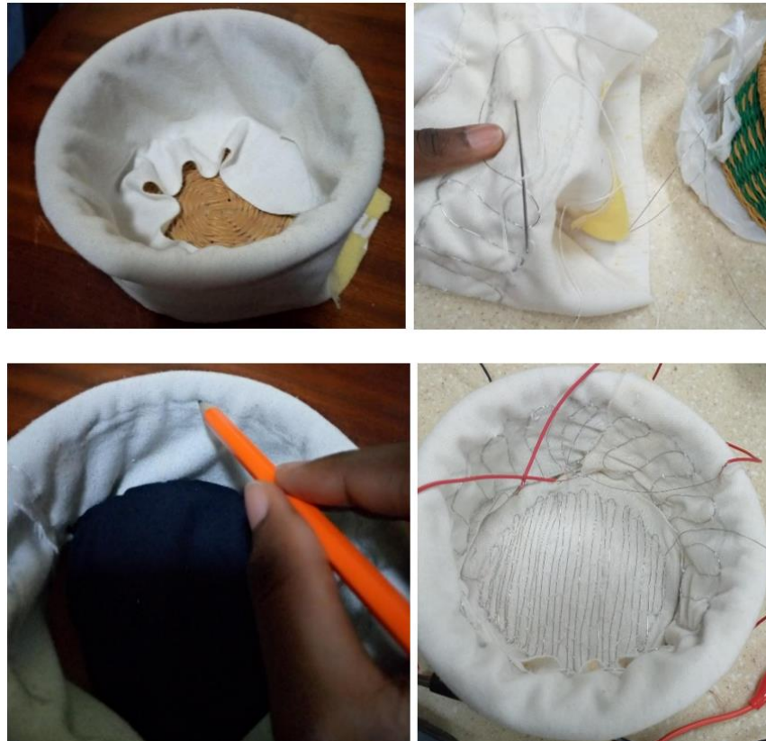
Figure 4.6: Captures of some stages in implementing the heating element
