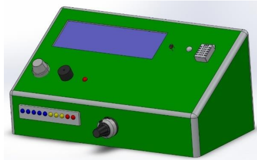
Figure 4.14: Modelled casing of the electronic components
