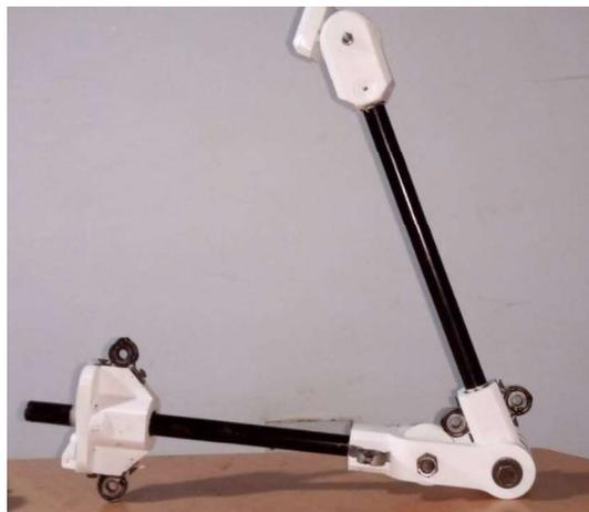
Figure 5.5: Fully jointed arm skeletal unit
