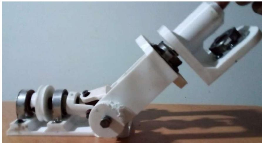
Figure 5.7: Assembled shoulder module side view with shoulder in abduction (elevated); (From left to right) Shoulder supporting bearings, Shoulder flexion/extension pulley on shoulder, Double cardan joint, Shoulder abduction/adduction socket, Shoulder
