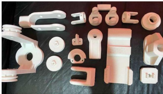
Figure 5.1: 3D-printed lightweight arm joint components
