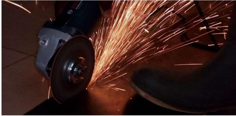
Figure 5.2: Sheet metal cutting of humanoid arm shoulder support and limbs
