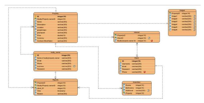
This shows the relationship between the entities of the Abode database, the primary keys and foreign key constraints. The diagram shows the attributes of the tables in the database.
