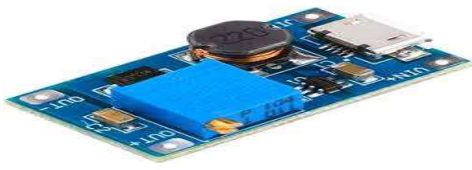
Figure 3.4 Boost converter and its schematic
