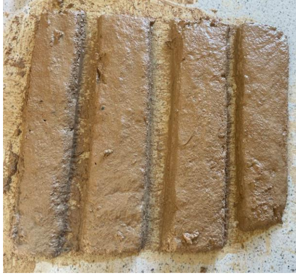
Figure 3.6: Selected Photograph of Freshly Applied Composite Slabs Before Molding and Forming Took Place
