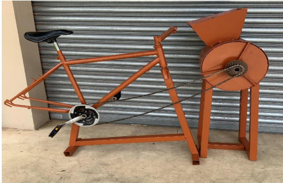
Figure 3. 2: The fabricated bicycled-power maize sheller [4]
