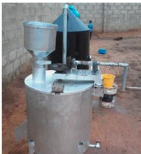
Figure 2.4: Shea nut kernel roaster [19].
