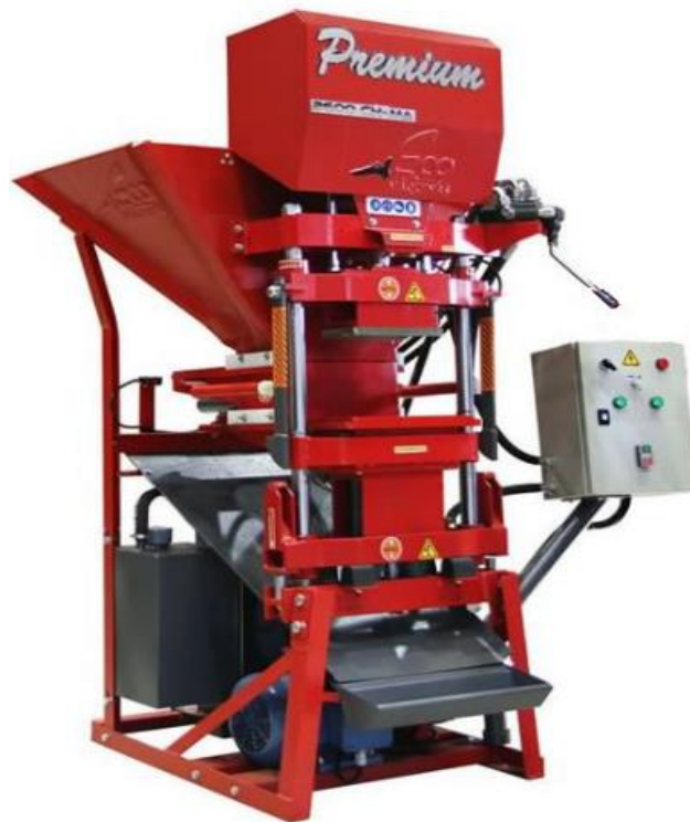
Figure 2 Semi-automated block making machine
