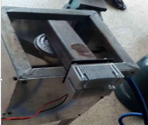
Figure 14 The heat probe placed on gas stove to test the TE generator
