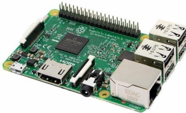
Figure 3.6.1 Raspberry Pi 3b
