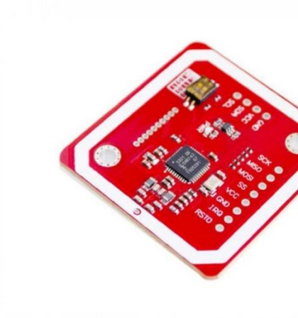
Figure 3.6.2 PN532 NFC module
