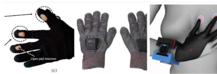
Figure 4.3.2.1 Open-pad structure, circuit kept at the back of the hand or worn on the wrist.
