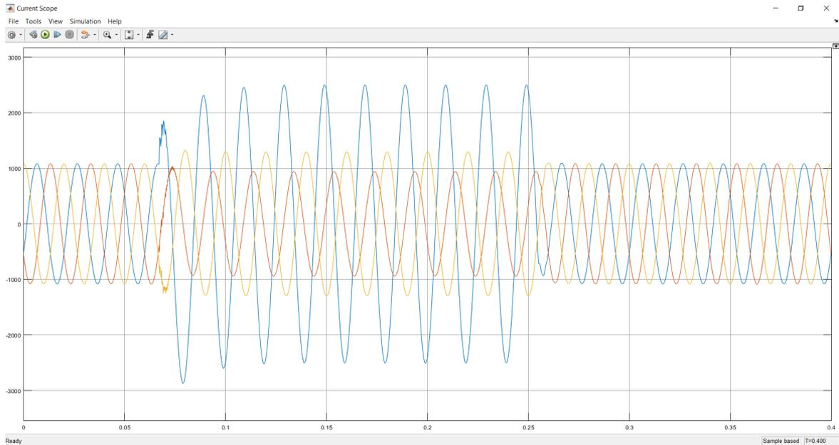
Figure 5.3: Current Output for a SLG fault
