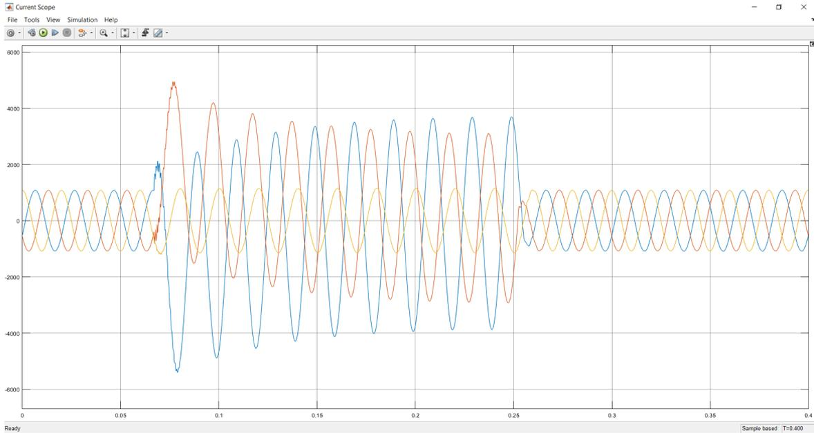
Figure 5.4: Current Output for a DLG fault
