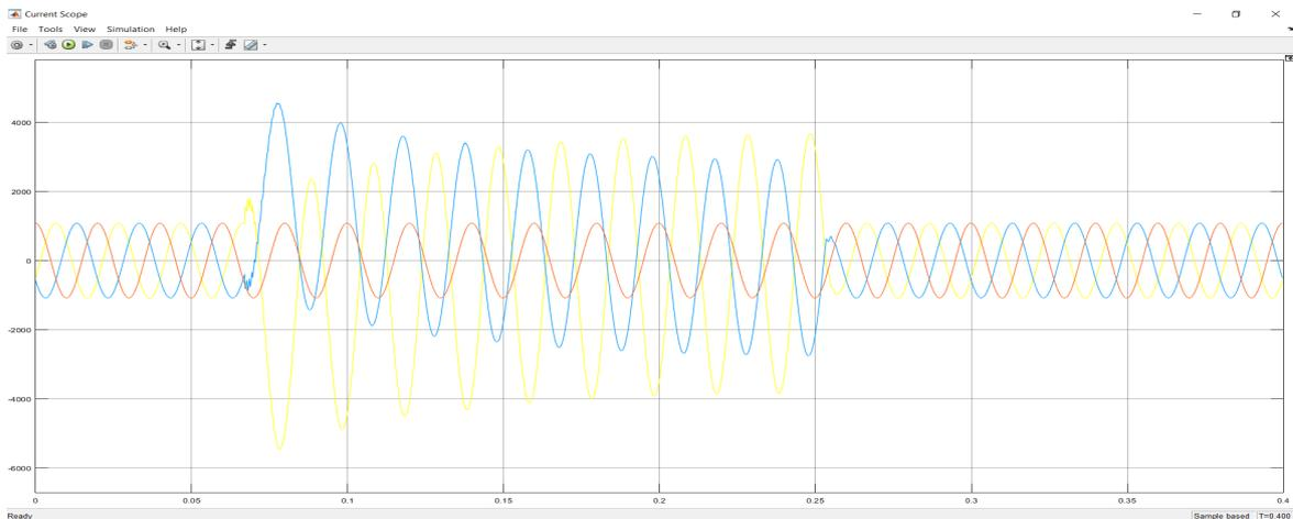
Figure 5.6: Current Output for a Line-Line Fault
