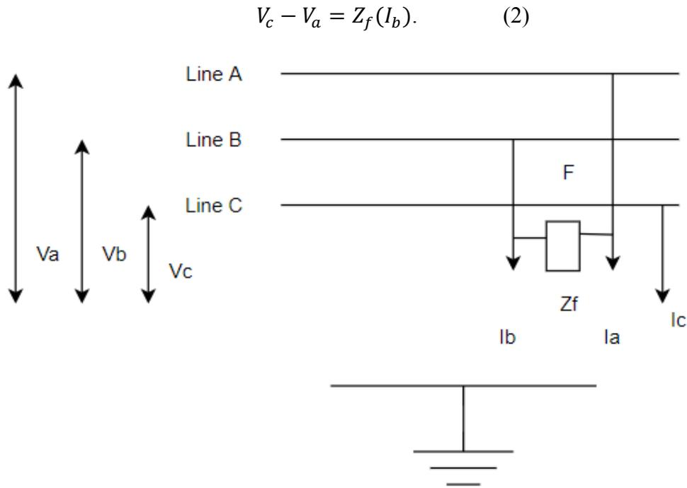
Figure 2.2 A diagram of Line to Line Fault
