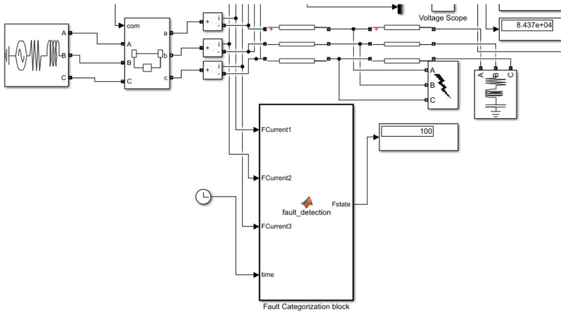
Figure 5.10: Diagram illustrating SLG Fault Categorization
