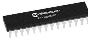
Figure 3.4: Microcontroller Atmega328
