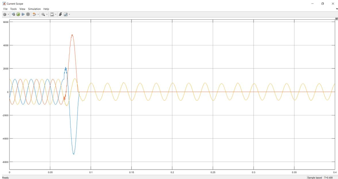
Figure 5.7: Current Output Showing isolation for a DLG Fault
