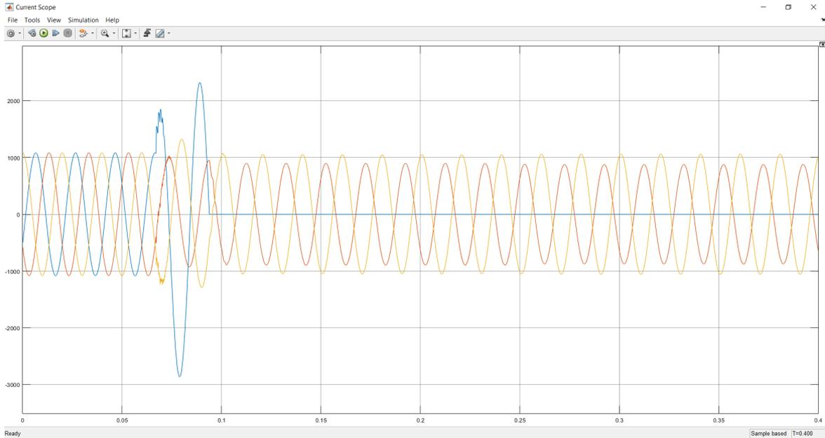
Figure 5.8: Current Output Showing isolation for a SLG Fault
