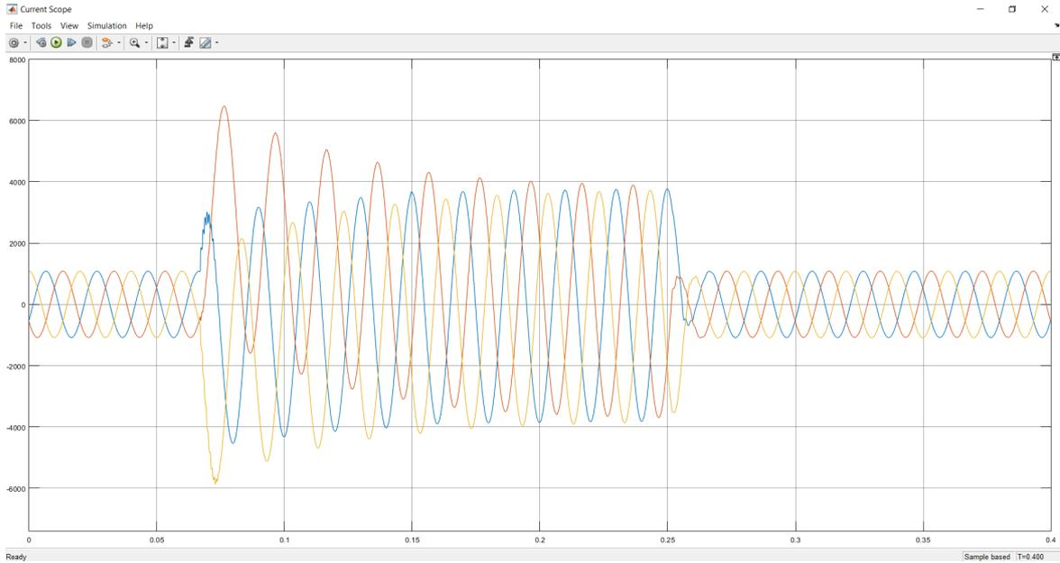
Figure 5.5: Current Output for a Three Phase to Ground Fault
