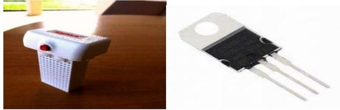
**Figure 14:** 2S ,7.4V ,2000mAh Li-ion UAV battery on the left, L7805 voltage regulator on the right
