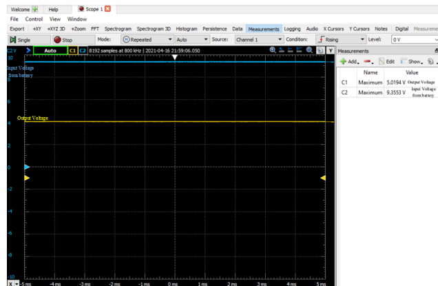
Figure 4 The digilent waveforms oscilloscope window showing the output and the input voltage
